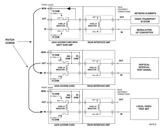
Figure 27. Non-Intrusive Insertion of Video Test Signal with Unity Gain Jack Access Card
